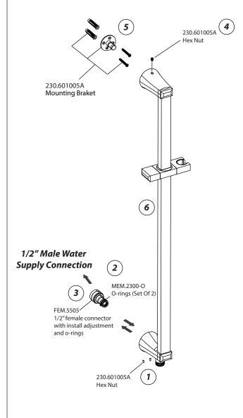
1. Loosen & remove two hex screws using 1.5mm Allen key.
